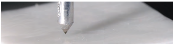
Surface roughness tests
